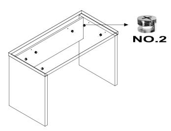
Step 4: Use NO. 2 to fix O4 with other parts and complete the installation.
