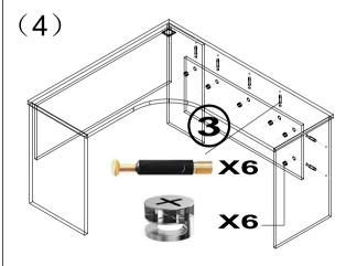
Step 4: Use A and B to connect ③ to other parts
