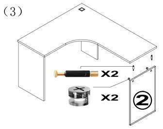
Step 4: Use A and B to connect ② to other parts
